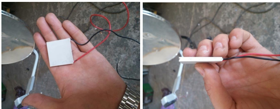
Figure 28: BiTe thermo electric cell module
