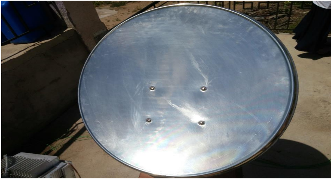
Figure 27: The solar parabolic dish reflective surface
