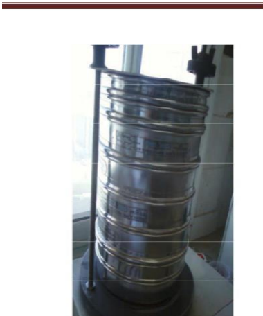
Plansifter with Sieve Particle Size .
