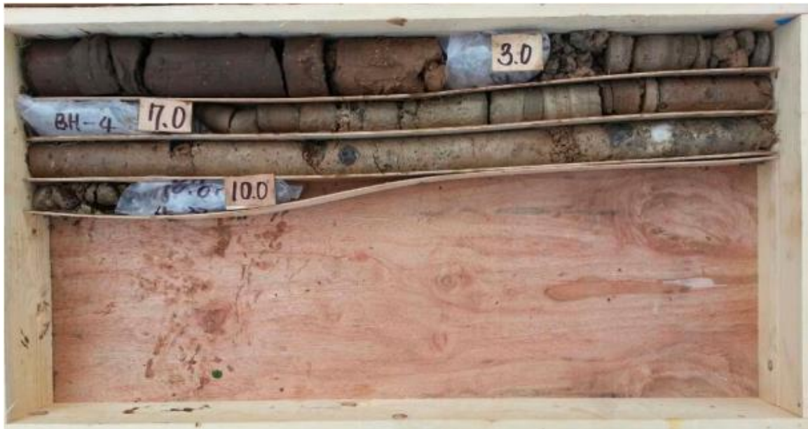
Figure III 1: Sondage carottés BH-04
