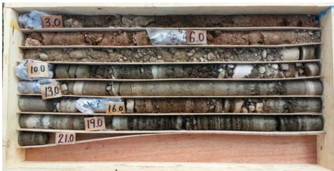
Figure III. 2: sondage carottés BH-05
