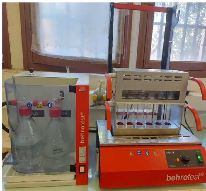
Figure 39mineralisateur kjeldahlbehrotest
