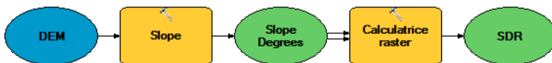
Figure 3.12: ArcGIS ModelBuilder workflow for integrating SDR into sediment yield estimation.
