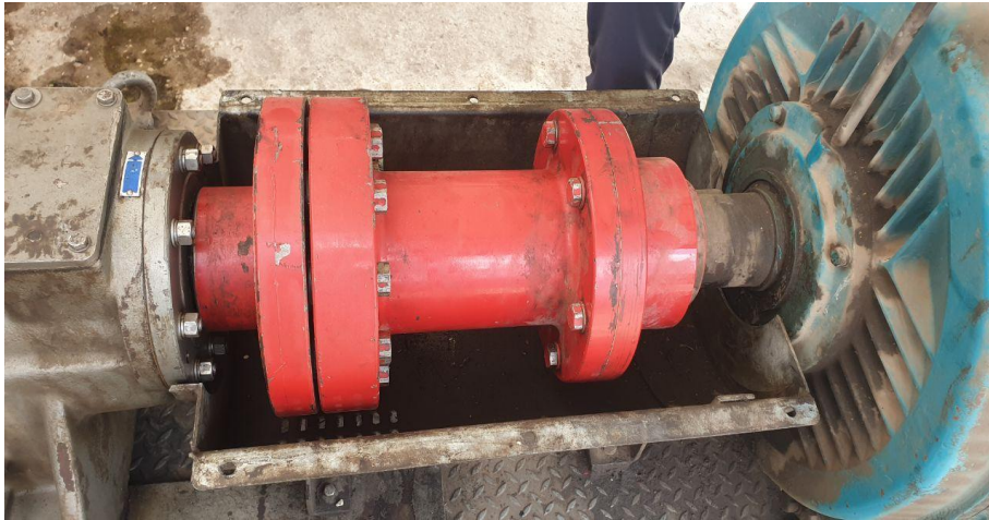
Figure 3-2 : Coupling sleeve connecting the motor shaft and the turbine shaft.
