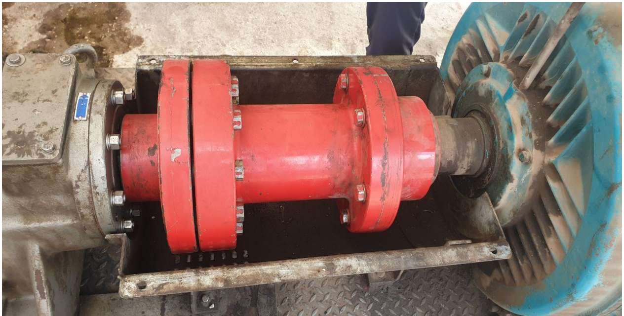
Figure 2-8: Schematic and Real View of Coupling
