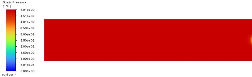
Figure 23 Pressure contour for methane-air combustion for global reaction at the equivalence ratio \Phi of 1
