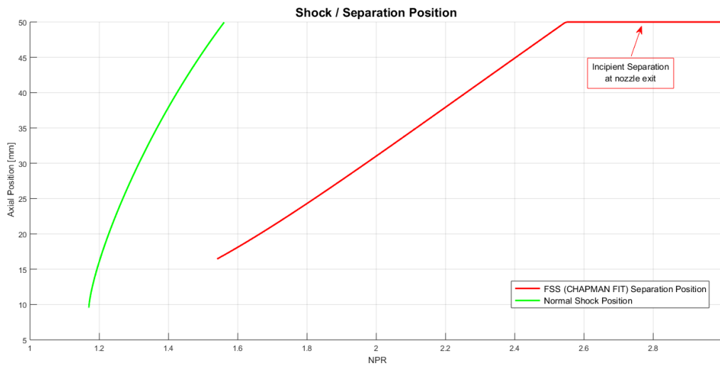
Figure B.4 : Normal shock/Separation position analysis.
