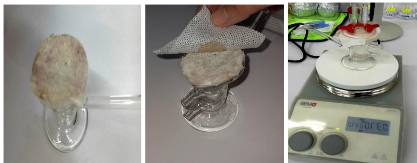
Figure 13: Stepwise assembly of the Franz cell diffusion
