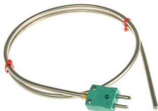
Figure 35. Photo de thermocouple. [40]
