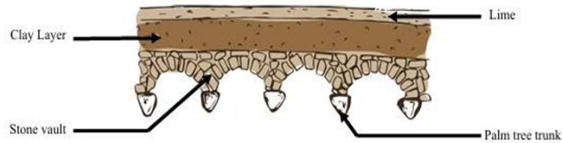
Figure 2.15: Section on a roof of palm tree trunks and vaults in the upstairs bedroom of the case study.
