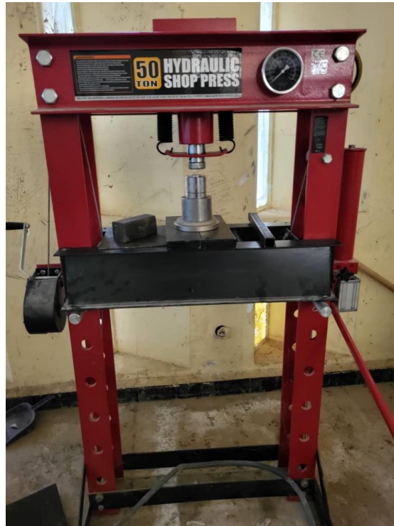
Figure 2.10 : Appareille de compactage "50-ton hydraulic shop press".
