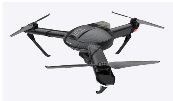
Figure 1.5: drone tri-rotor [16]
