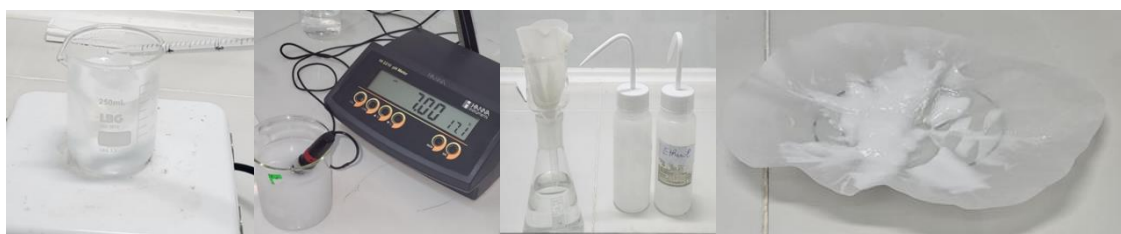
Figure III.6: steps for the preparation of ZnO nanoparticles.
