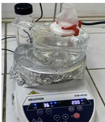
Figure III.8 : Franz Diffusion Cell Setup
