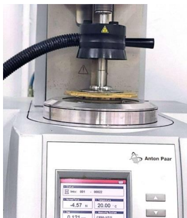
Figure III.7: Rheological measurements were conducted using a cone-plate system.
