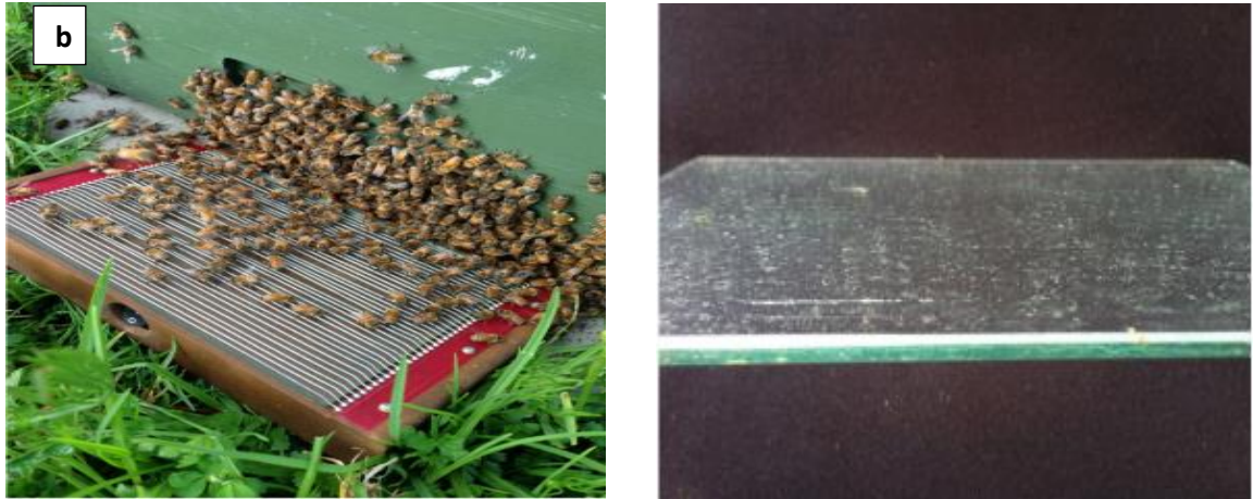
Figure 1.1. Bee venom collector Bee whisper 5.0 is based on the electric stimulation protocol In (a) it is shown how the equipment is put in front of the hive entrance. After completion of the collection cycle, the venom that has been deposited on the glass slide (b) can be scraped down. [9]
