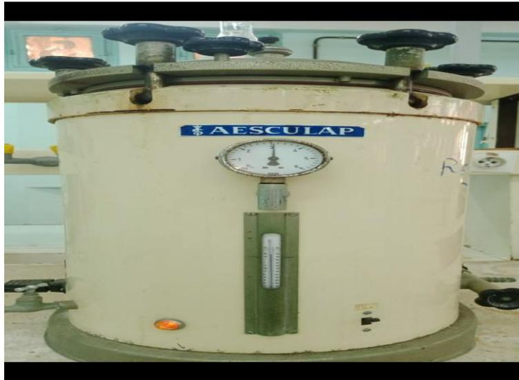
Figure 2.5 : Autoclave.
