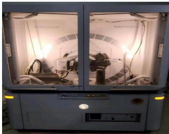
**Figure II.5:** Diffraction Des Rayons X
