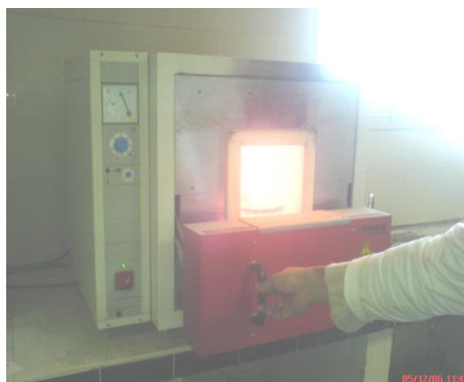
Figure III.2. Four a moufle ( T_{\text{max}} = 1250\text{ }^\circ\text{C} )
