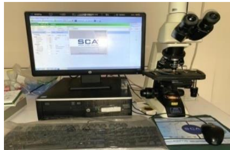
Figure 19 : Système CASA (Computer Analyser System Assisted) (Photo originale).
