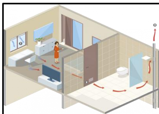
Figure 7: ventilation naturelle Source : Architecture et climat 2023
