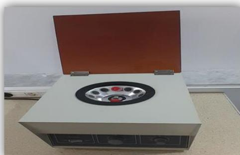
Figure 9: centrifugeuse des tubes sanguins(Hadj-Arab,2025)
