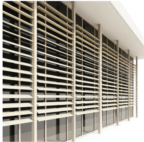
Figure 3.83: Facade that shows horizontal louvres. Source: authors, enhanced by AI.
