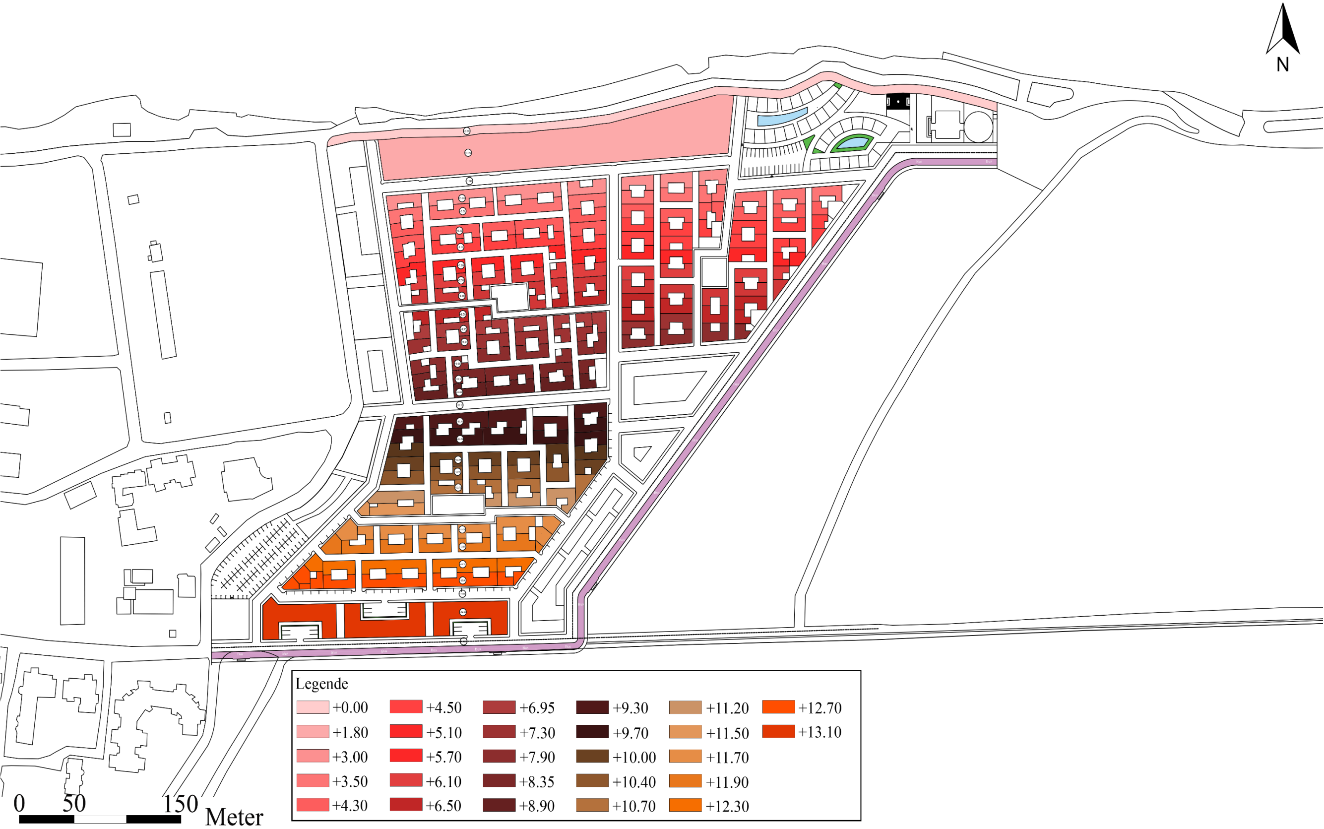
Figure 59: Spot Elevation Plan, Source: Author, Software : AutoCAD, Treaty by Software: photoshop.
