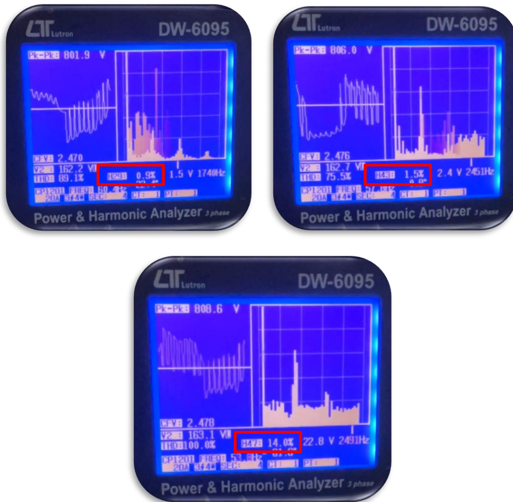
Figure (III.45) : Analyse spectrale FFT (THD)
