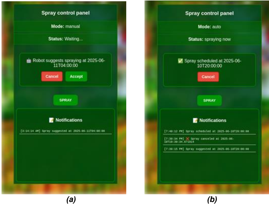
Figure 4.3: Spray control panel showing (a) a user prompt in Manual Mode and (b) an automatically scheduled spray in Auto Mode.
