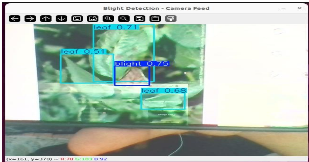
Figure 4.9: Real-time Detections by the YOLOv8n Model Showing Late Blight and General Good Detection
