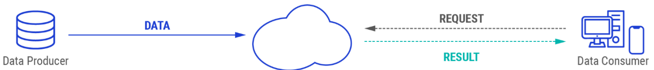
Figure 1.1: Conventional cloud computing structure.
