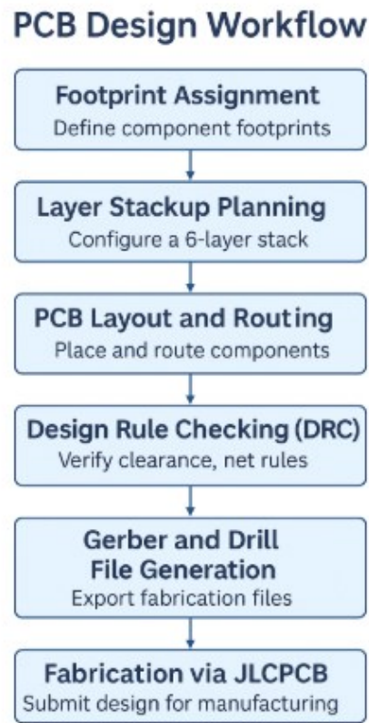
Figure 3.14: PCB Design Workflow from Schematic to Fabrication
