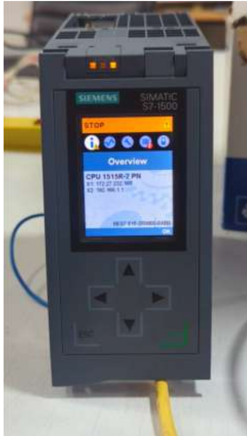
Figure 1. 8: automate Siemens S7-1500 [15]
