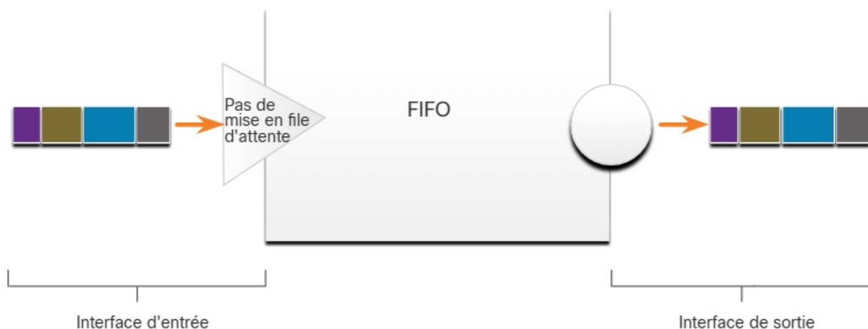
FIG. 3.3: FIFO(First In, First Out)– Source : [31]
