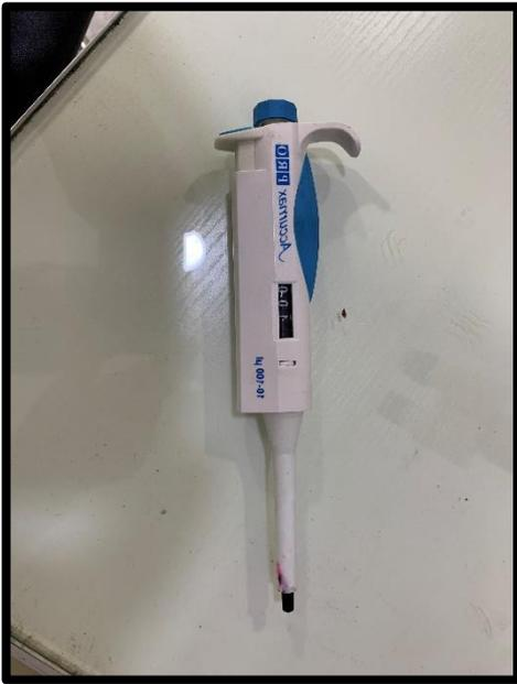
Figure 45 : Micropipette graduée 10 - 100 $\mu$
