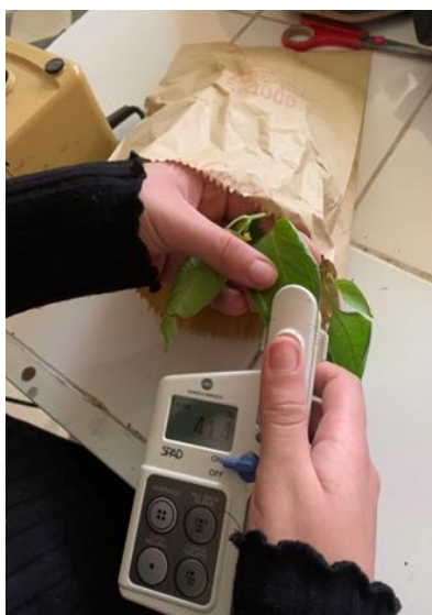
Figure 15: Measurement of chlorophyll content using a chlorophyll meter (Original, 2025)
