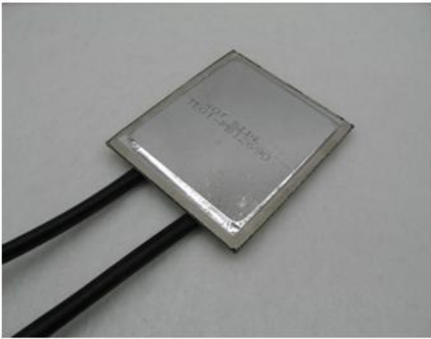
Figure 3.1: Lead telluride (pbte) Thermoelectric generator
