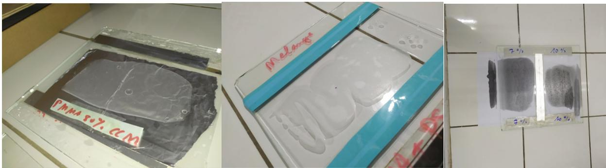
Figure 2-4 : Formation des films composites PMMA/PSU/graphite.
