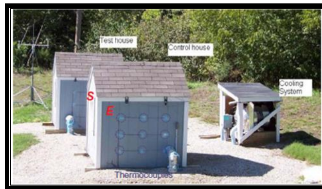
Figure 2. 7. Image des cabanes de test [210]
