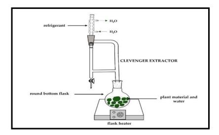
Figure 6: Schematic representation of hydro distillation (Sousa, V.I et al., 2022)
