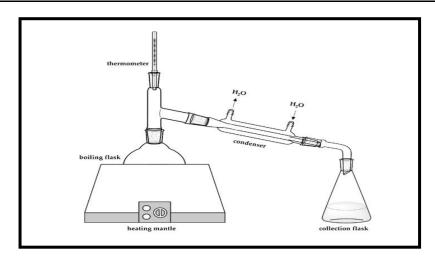
Figure 7: Experimental setup used in stream distillation (Sousa, V.I et al., 2022)
