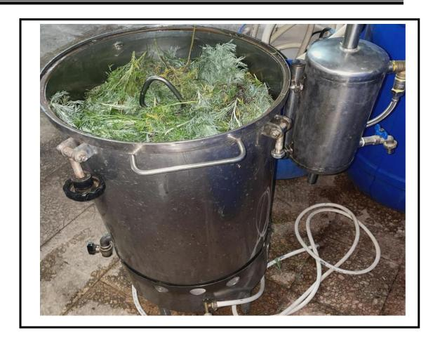
Figue 18: Alembic-type apparatus with a 50-liter capacity (original photo)
