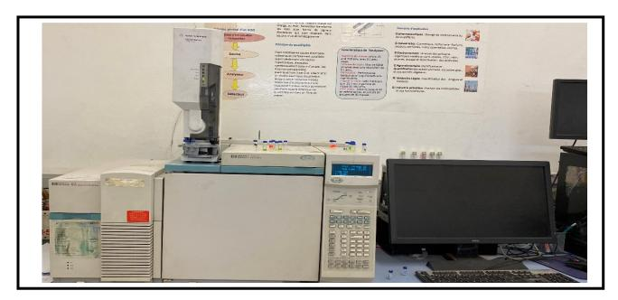
Figure 20: Hewlett Packard GCMS- Agilent 6890 instrument (original photo X).
