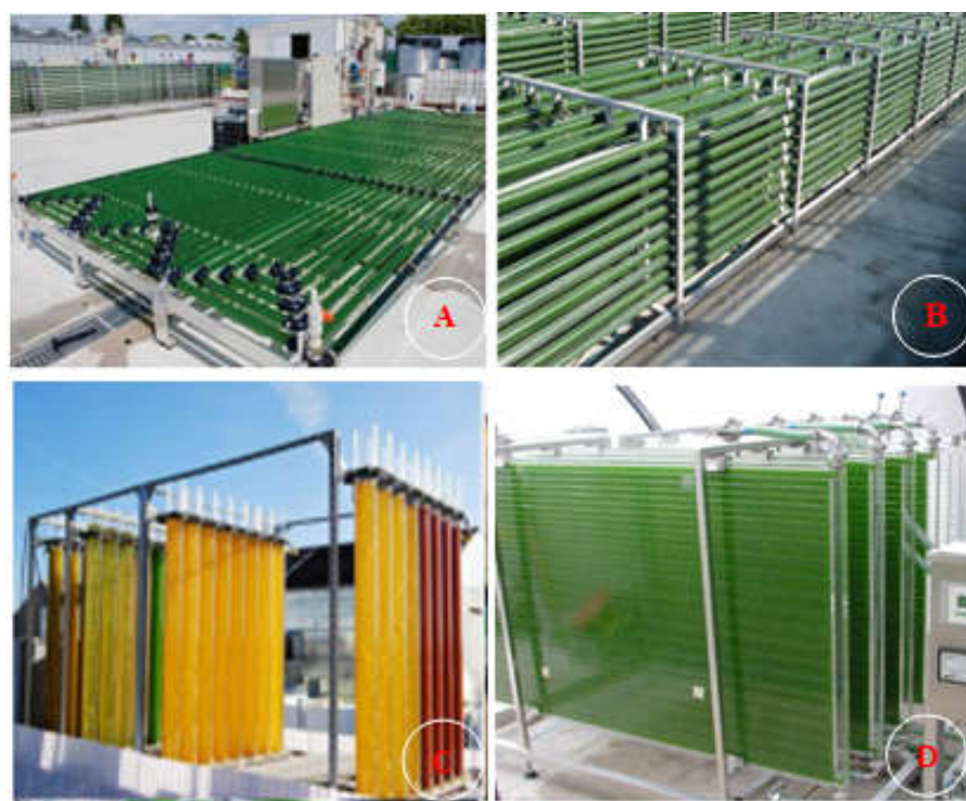
Figure 2. Different culture types of closed system; (A) Horizontal tubular reactors (Pereira et al. , 2018). (B) Vertical tubular reactors (Devi et al. , 2013), (C) vertical column reactors, (D) Flat panel reactors (Jerney & Spilling, 2018).
