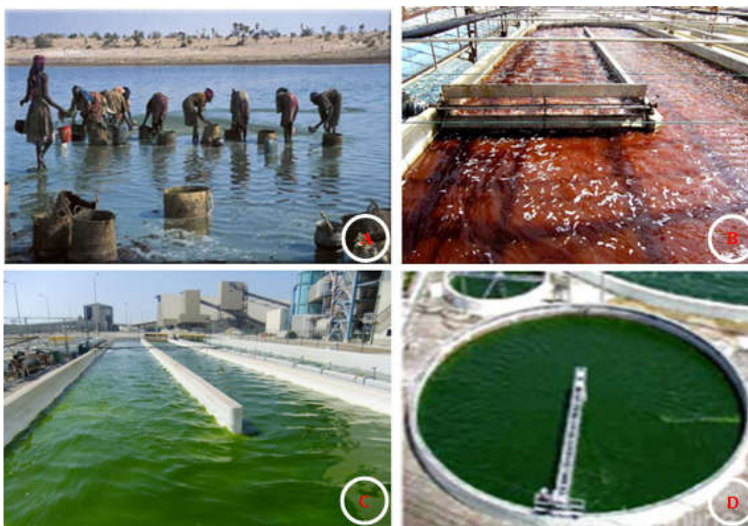
Figure 1. Different culture types of open system for microalgae production (A) Kanembu women harvesting Spirulina from Lake Boudou Andja, in Chad. (Hamed 2016), (B) Production of Haematococcus in raceway pond (Zhang al. , 2009), (C) Production of microalgae in raceway pond, (D) Microalgae mass production in circular pond (Shen et al., 2009).
