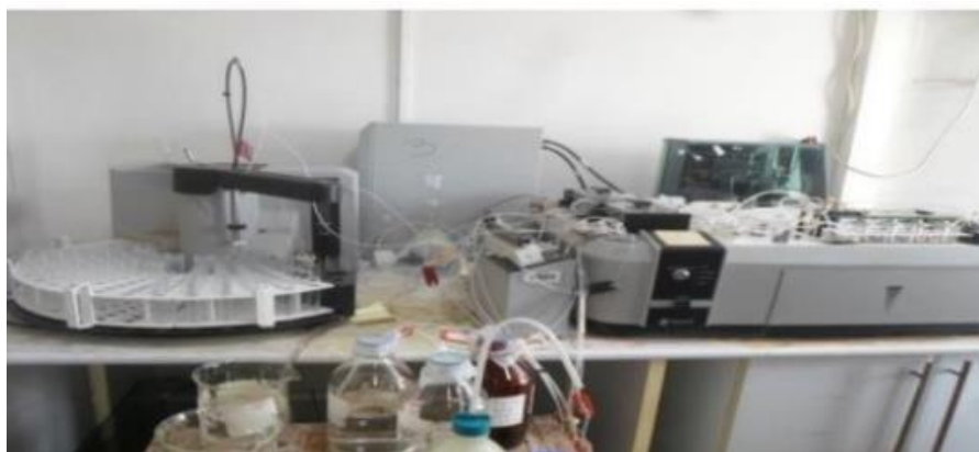
Figure 3.8: Continuous flow analyzer (central laboratory SEAAL, Algiers).
