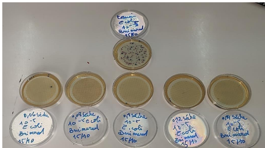
Figure 4.48: Treated samples and witness (case of E. coli and coliforms) using ferrate (VI) (Beni Mered WWTP).
