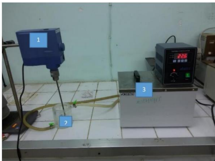
Figure 3.2: Experimental setup used for the synthesis of ferrates by the dry route. 1- Mechanical stirrer, 2-Double-walled electrochemical cell, 3-Water bath.
