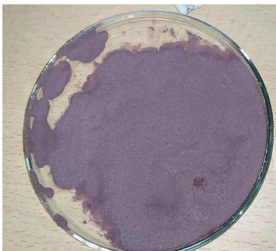
Figure 4.21: Potassium sulfate ferrate (VI) after drying
