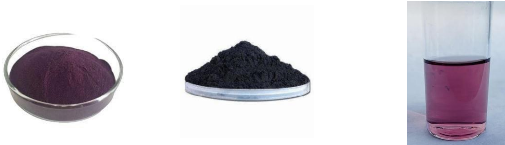
Figure 1.4: Ferrate (VI) color in powder form and in aqueous solution.
