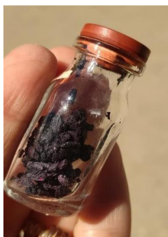
Figure 4.28: Sodium ferrate (VI) powder synthesized with electrochemical method.
