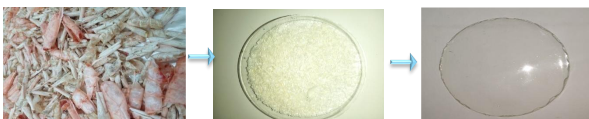
Figure 4.1: From red shrimp shells to chitosan membrane.
