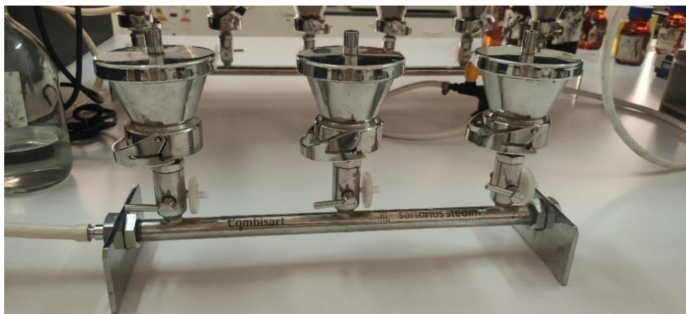
Figure 3.10: bacterial filtration system (microbiology laboratory, SEAAL).
