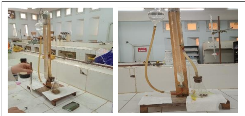
Figure 17: Dosage du calcaire total (Original 2025).
