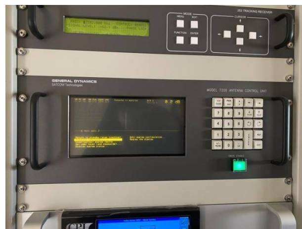
Figure II.5 : Antenna Control Unit ( ACU )
