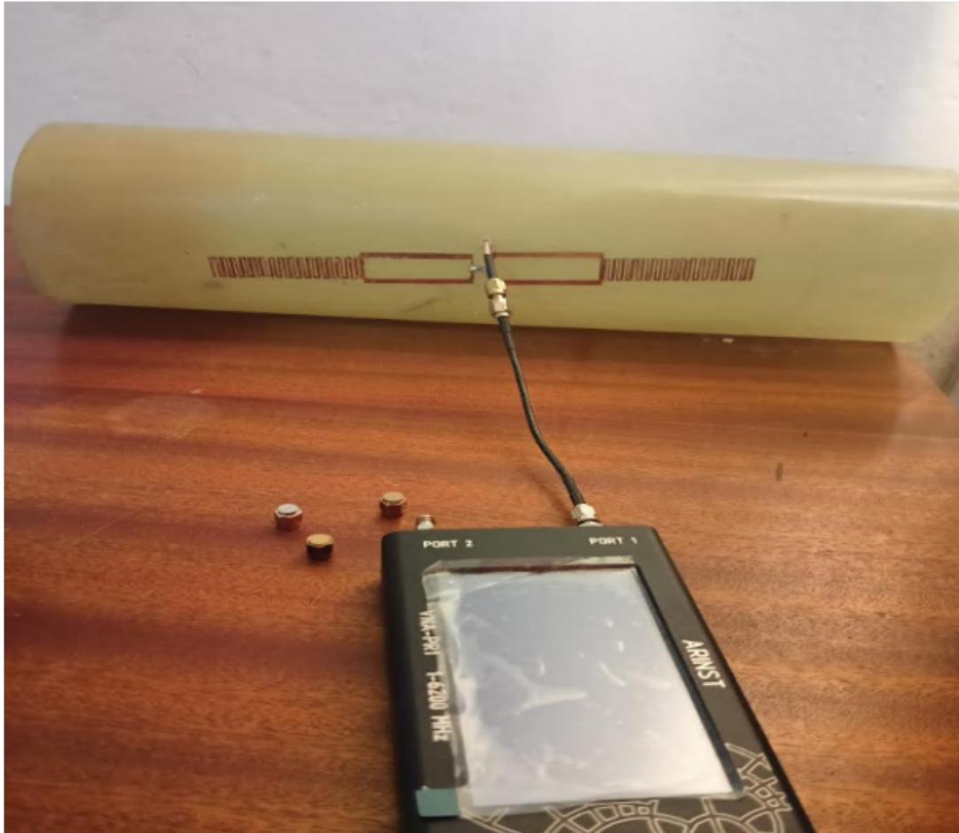
Figure 3.26: Antenna to VNA interface for measurement
