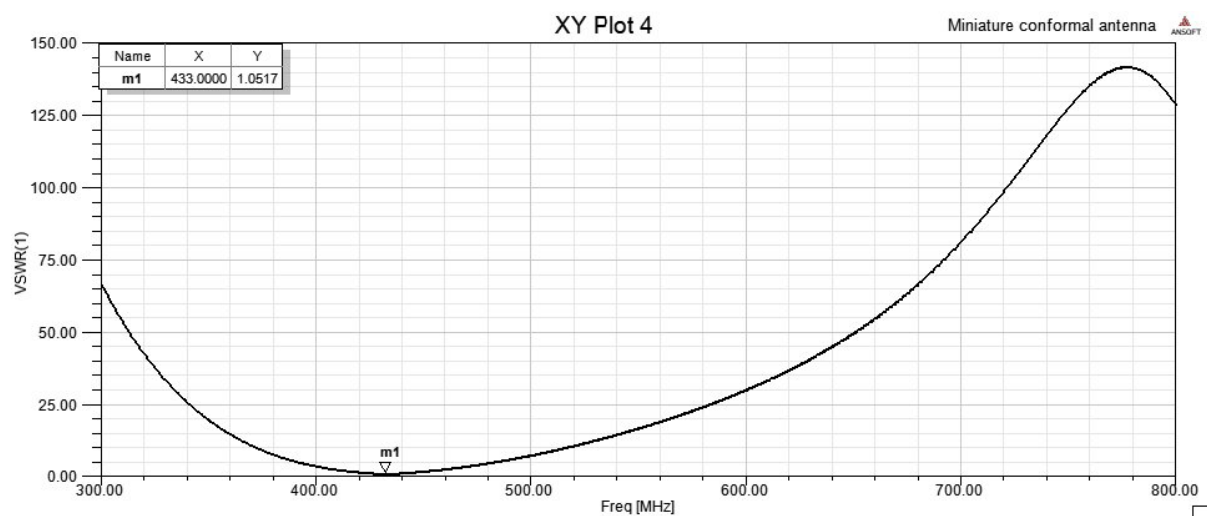
Figure 3.16: VSWR characteristics of the optimized miniature antenna
