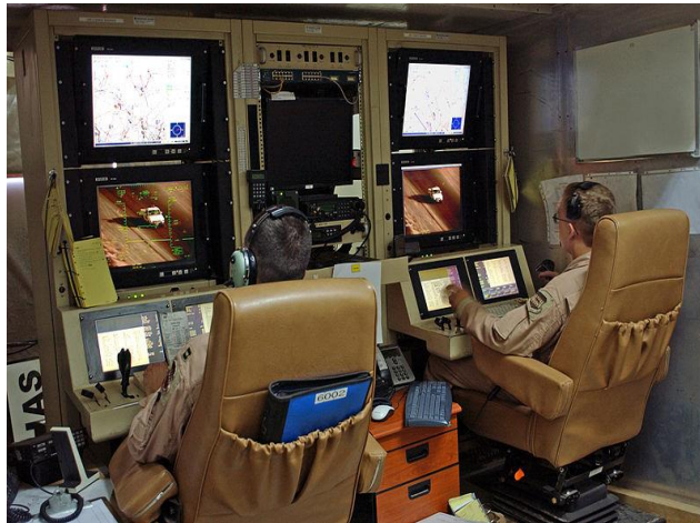
FIG.I.1 Station au sol. [4]
