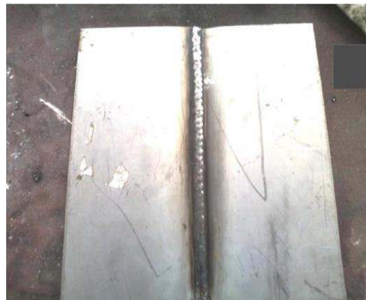
Figure III.1. Microstructure de l'acier 316L. Figure. III.2. Acier inox 316L soudé.
