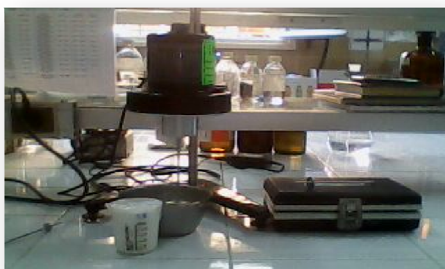
Figure 13: Viscosimètre : Customer calibration record "mobile 7"
