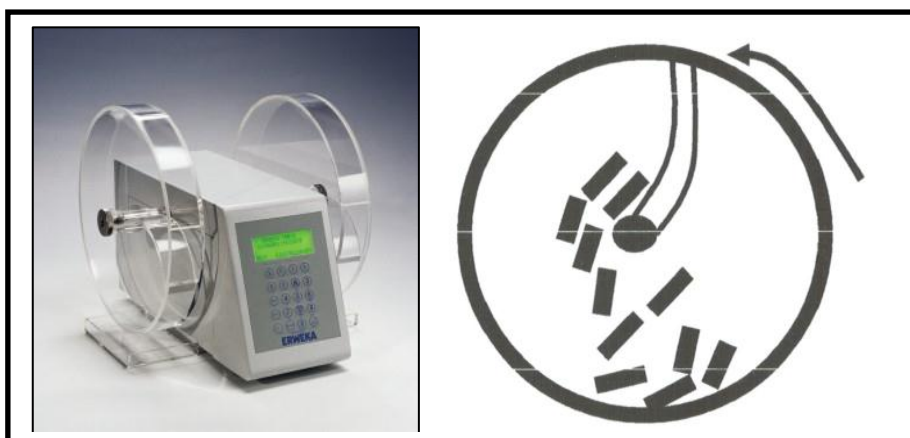
Figure II.12: photo Friabilimetre (ERWEKA).
