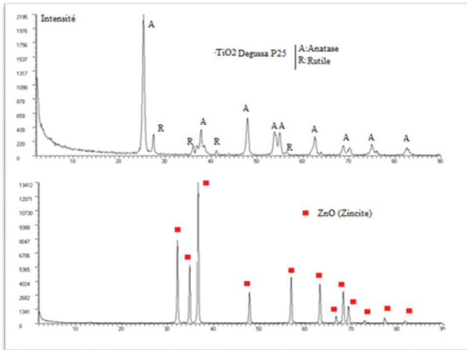
Spectre de diffraction RX du  $\text{TiO}_2$ , ZnO.
