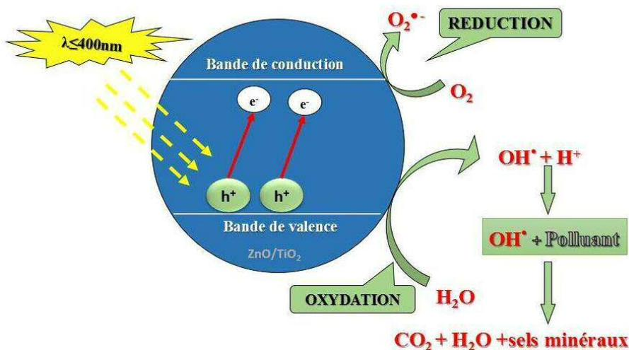
Figure I.2: principe de la photocatalyse
