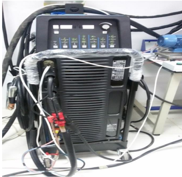
Figure 04: photo du poste de soudage Miller Dynasty 350,700 Maxstar 350,700.
