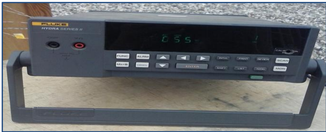
Figure III.1 : Photo de l'acquisition des thermocouples.
