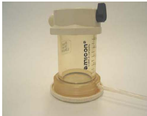
Figure III. 3 Cellule Amicon de filtration frontale (Amicon-Millipore)
