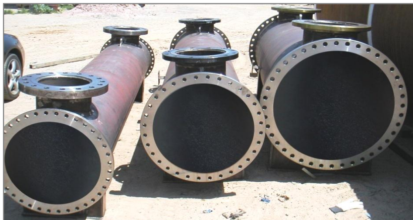
Figure II.7 : calandre type E (une passe) [14].
