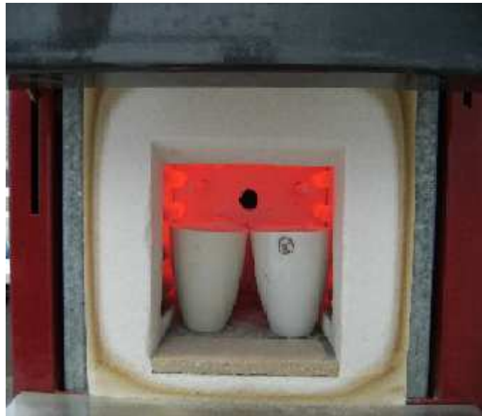
Figure 2.7: Calcination du kaolin
