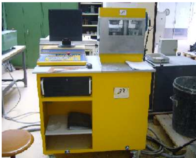
Figure 2.9: Machine de compression/flexion 3R.
