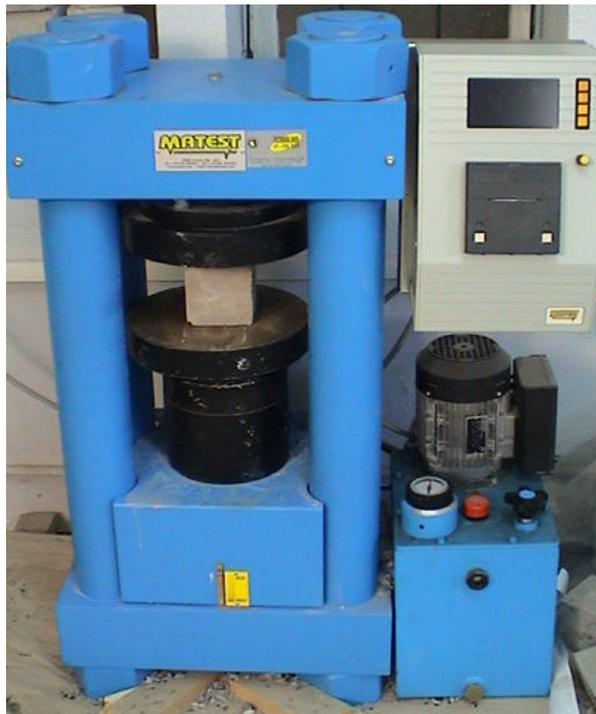
Figure 3.18: Essai de compression simple.
